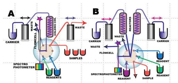
The sample port has an inlet and outlet which meet on the face of the COV rotor. Thus the sample can be primed to the valve without drawing sample into the rest of the manifold where it can cause carryover. The sample port can also be primed with the next sample while the present measurement is underway by using the second milliGAT pump (A) or miniaturized metering pump.
